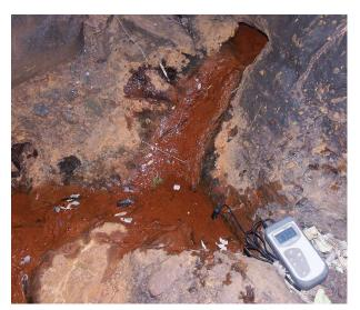
Photo KG080089, Measuring electrical conductivity in a seep at Widdallion Cave. The orange flocculated "mud" had an interesting chemistry (see Appendix 7 and section 4.1.5, on speleothems).
