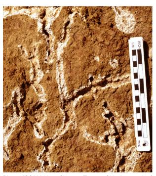
Photo KGS880107a, Charters Towers, Qld. A network of solution tubelets in laterite.
